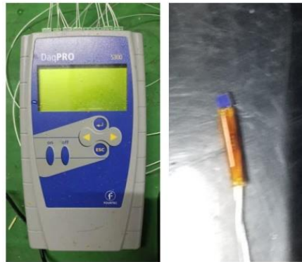
Figure 11. Temperature scanning valve and thin-film platinum resistance.
