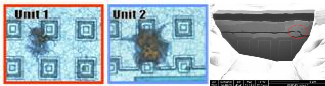
Fig. 2. Damaged metallization manifestation
