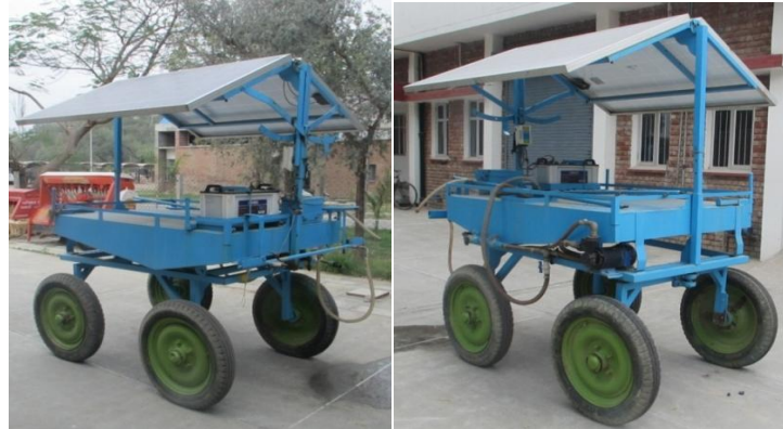
Fig. 3. Front and rear view of developed experimental machine
