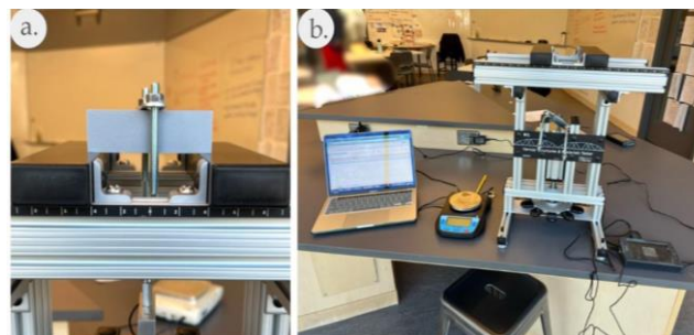
Fig. 4a. Example of test model loaded into the VSMT for data-gathering
