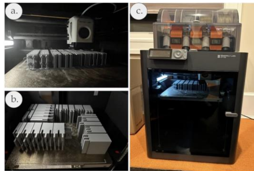
Fig. 2a. Inside of printer midway through printing models Fig. 2b. Models on build plate after finishing print Fig. 2c. Bambu Lab P1S used to print the models
