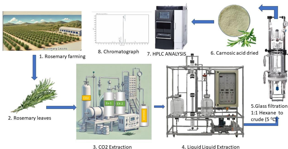
Fig. 1. Process flow chart of Super Critical CO 2 extraction of Carnosic acid from Rosemary Leaves
