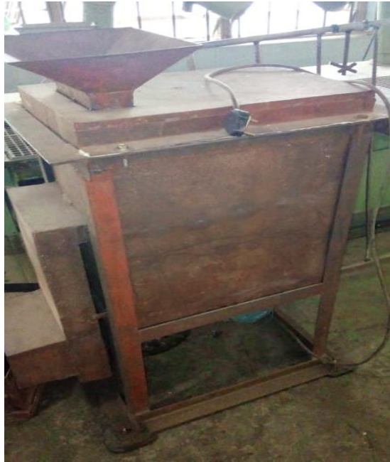
Fig. 6. The modified rice de-stoner
