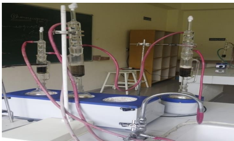
Fig. 2. Soxhlet assembly for extraction
