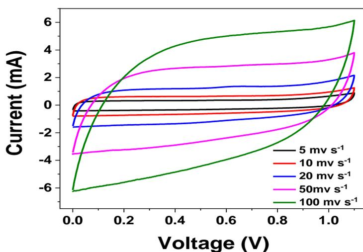
**Fig. 5. Cyclic voltametry (CV) of Na<sub>2</sub>S<sub>2</sub>O<sub>3</sub> activated cassava peel with 5 mvs<sup>-1</sup> to 100 mvs<sup>-1</sup> scan rates**
