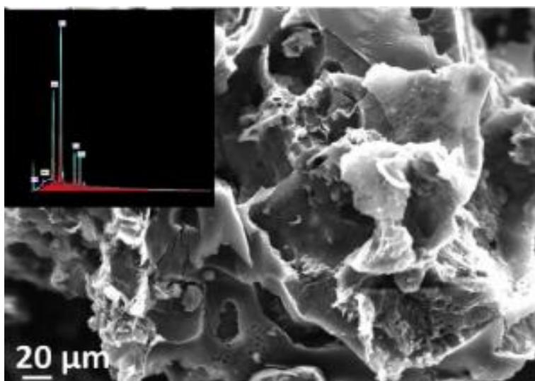
Fig. 3. SEM micrograph of the produced activated carbon with figure inset showing the EDX pattern of elemental composition
