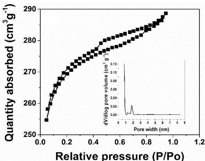
Fig. 4. Gas adsorption/desorption isotherms of  $\text{Na}_2\text{S}_2\text{O}_3$  activated carbon. Inset to the figure shows the BJH pore size distribution
