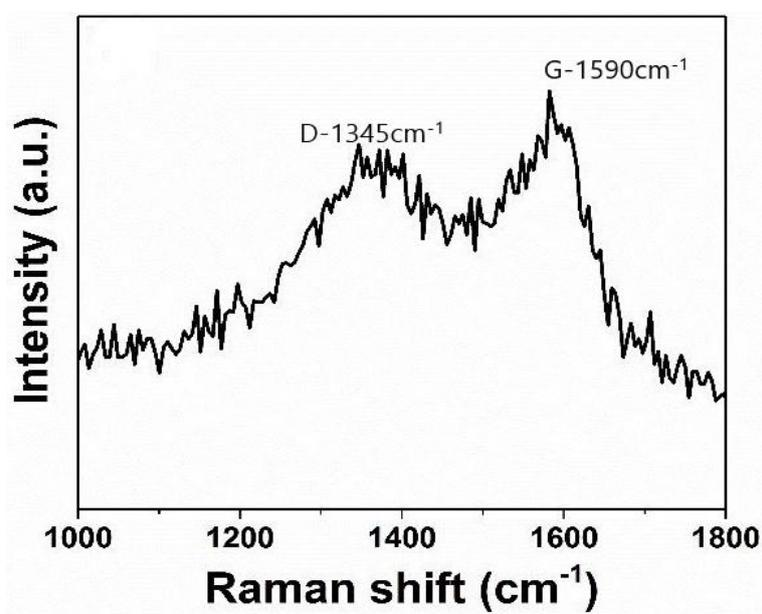
Fig. 2. Raman spectrum of the produced carbon material
