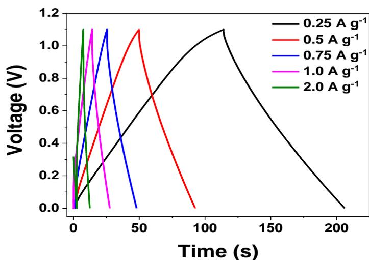
**Fig. 6. Galvanostatic charge discharge (GCD) of Na<sub>2</sub>S<sub>2</sub>O<sub>3</sub> activated cassava peel at 0.5Ag<sup>-1</sup> to 2.0Ag<sup>-1</sup> specific current rates**
