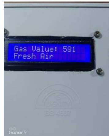
Fig. 10. Result screen of air quality monitoring system in ppm
