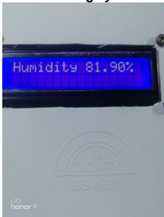
Fig. 9. Data of relative humidity on LCD Screen
