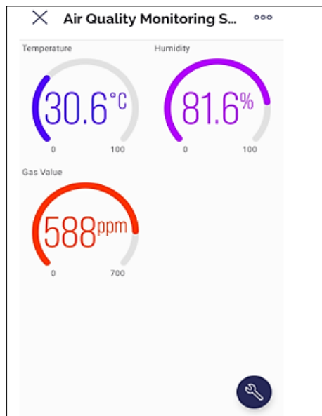
Fig. 11. Data of temperature, relative humidity and air quality on mobile app
