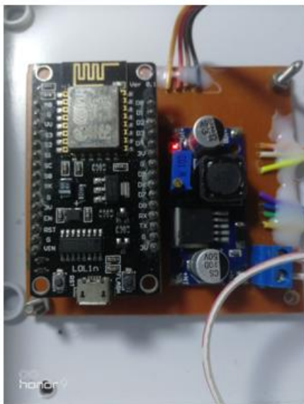
Fig. 5. Inside view of the air quality system
