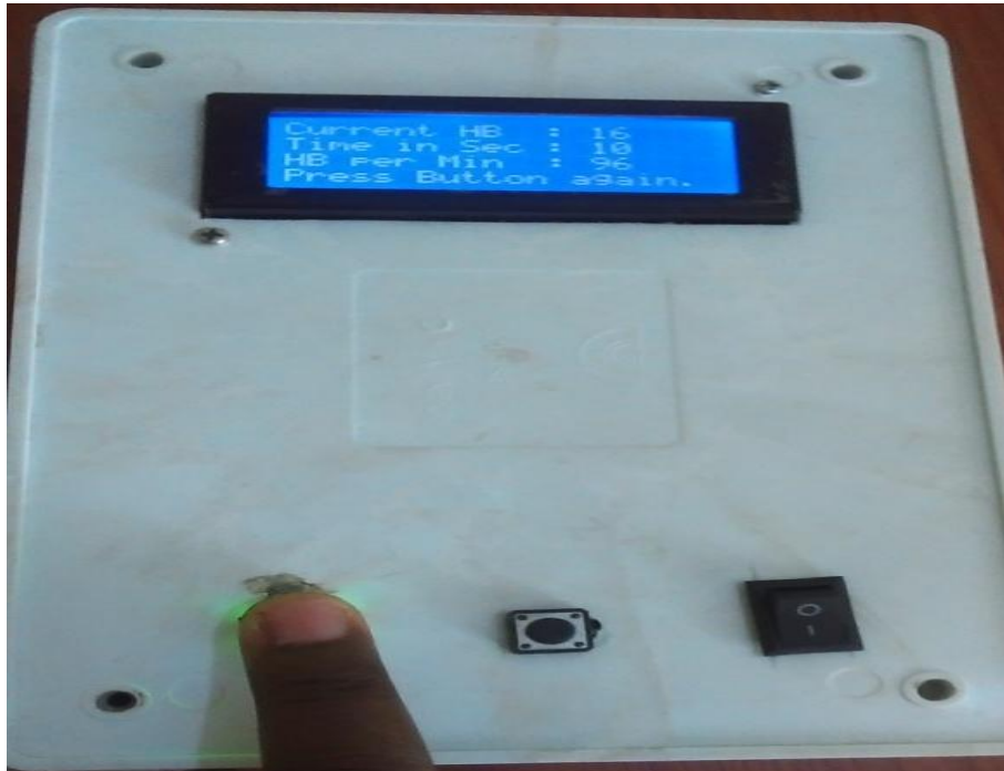
Fig. 13. Testing of heart beat by placing any finger-tip on sensor
