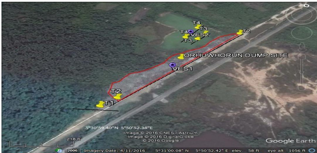
Fig. 4. Satellite Image of Orhuwhorun dump site with profile lines and VES locations
