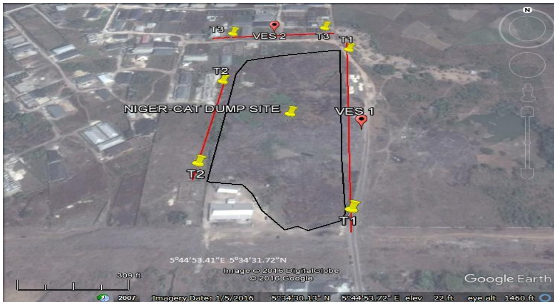
Fig. 2. Satellite image of Niger-Cat dump site with profile lines and VES locations
