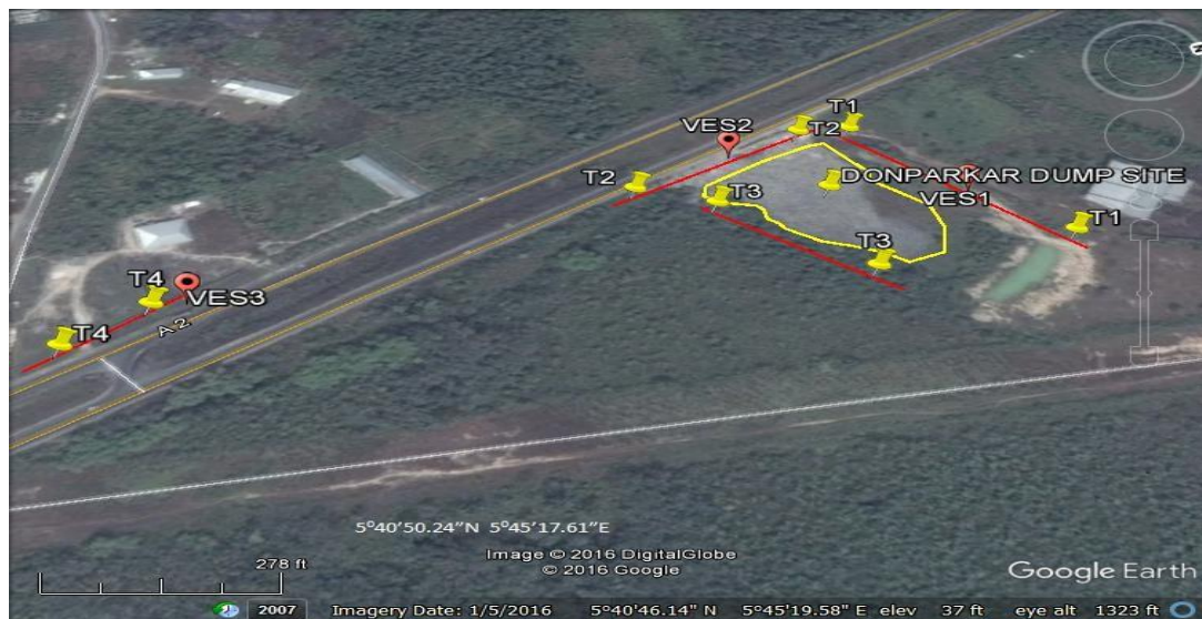
Fig. 3. Satellite image of Don-Parkar dump site with profile lines and VES locations
