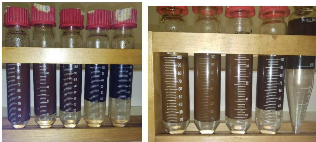
Appendix 4. Plates showing bottle test results for effective demulsifiers in Butanol at 60°C
