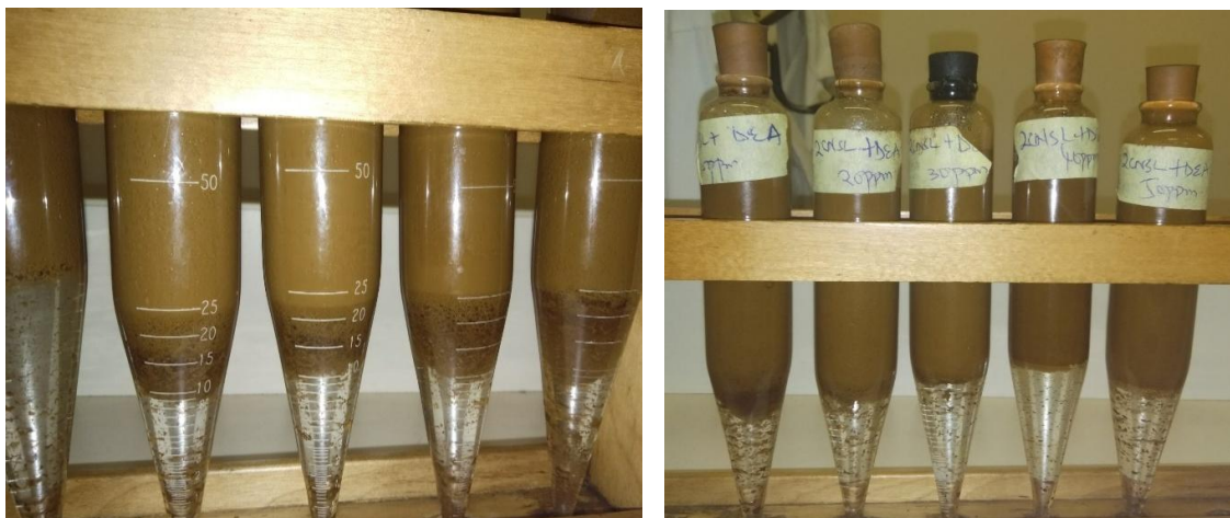
Appendix 4. Plates showing bottle test results for effective demulsifiers in Butanol at 60°C
