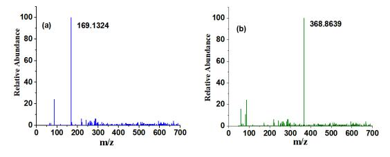
Fig. 5. ESI-Mass spectra of the (a) ligand, L and (b) [CuL(CH<sub>3</sub>COO)<sub>2</sub>(H<sub>2</sub>O)]
