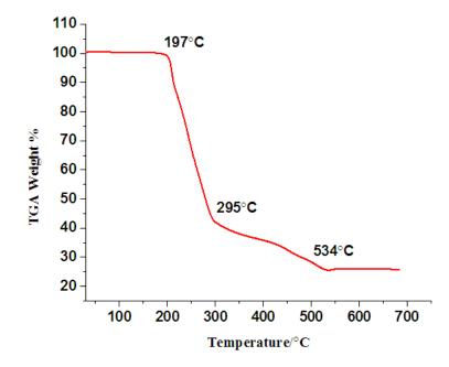
Fig. 6. Thermogravimetric (TG) curve for the complex, [CuL(CH<sub>3</sub>COO)<sub>2</sub>(H<sub>2</sub>O)]
