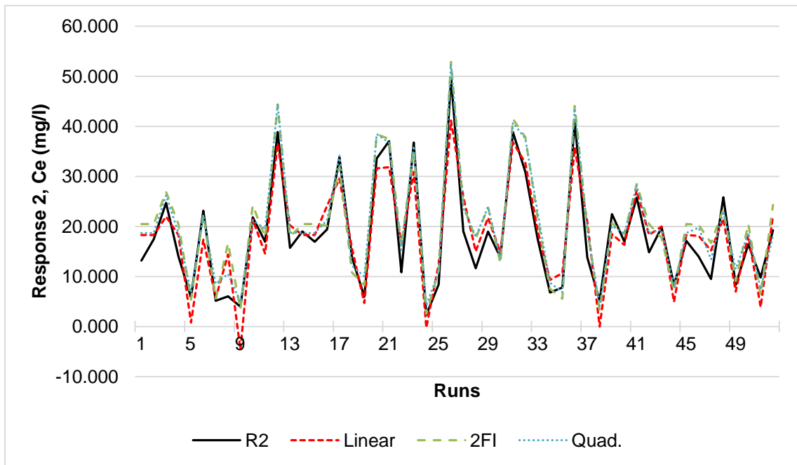
Fig. 4. Comparative plot of predicted R2 of all 3 RSM models studied and actual R2
