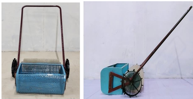
Fig. 5. Mechanical type neem fruit picker collector
