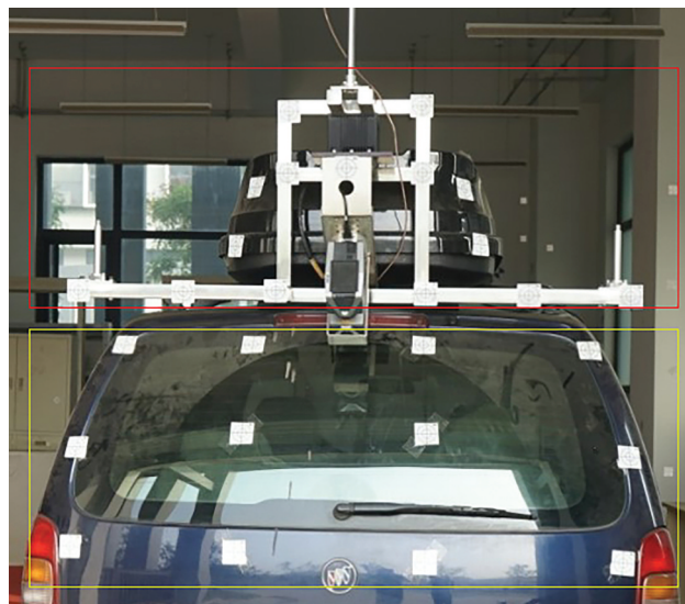
Figure 3. The layout of reflectors around MMS: A total of 27 reflectors are pasted on the MMS, among them, the red box is the verification point, and the yellow box is the control point.
